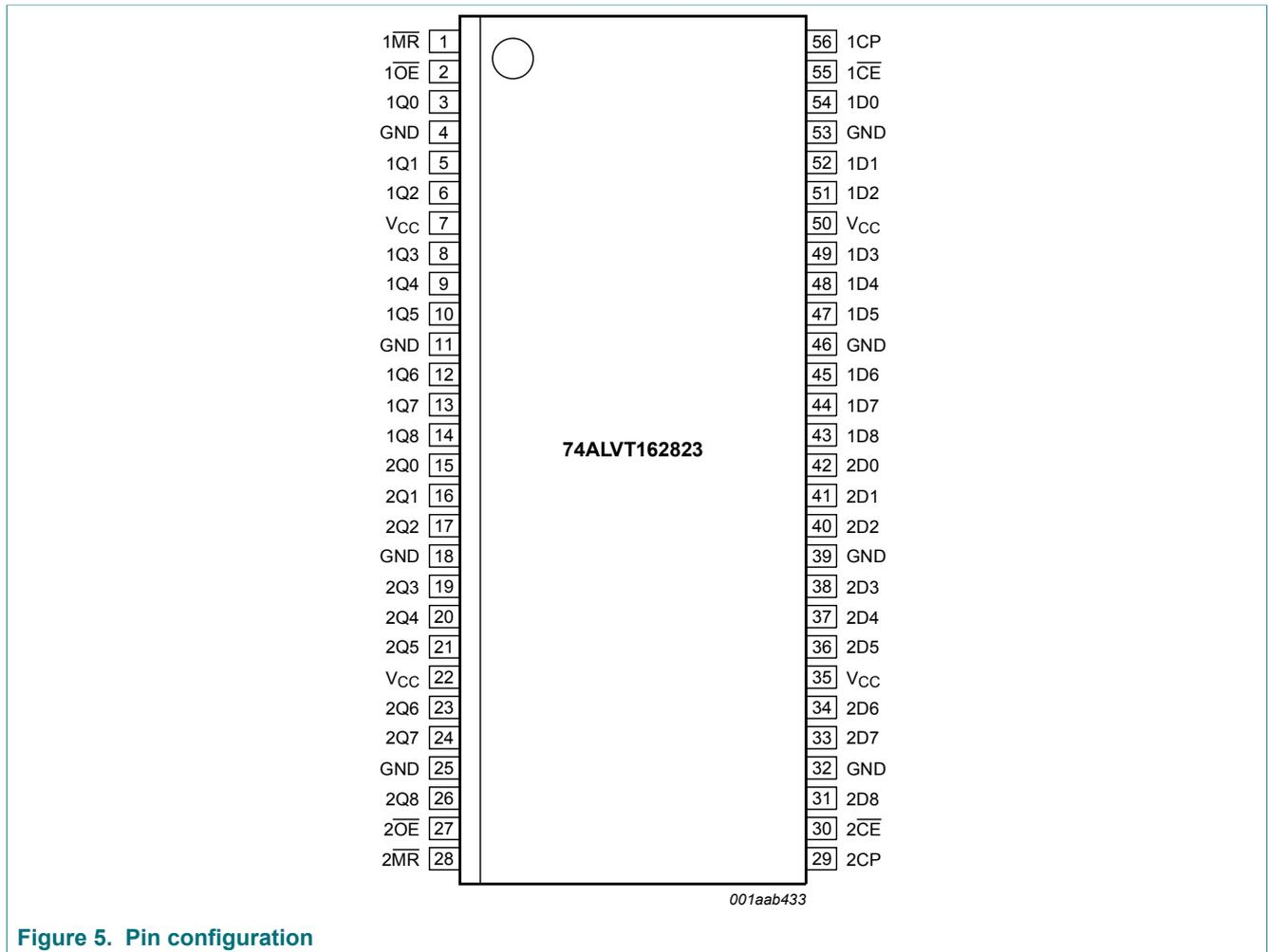
Figure 5. Pin configuration
