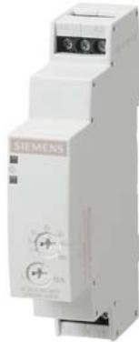
Timing relay, electronic OFF delay without control signal, 1 change-over contact 7 time ranges 0.05...100 s 12-240 V AC/DC with LED, Screw terminal
