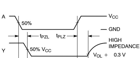
Figure 4. Switching Waveforms
