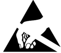
***Make it a habit always to first touch the mounting hole (which is grounded) for a few seconds with both hands before touching any other parts of the boards.*** That way, you will have the same potential as the board and therefore minimize the risk for ESD.
