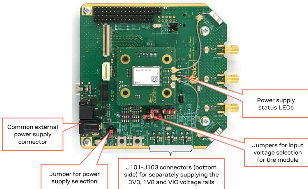
Figure 7: Overview of EVB power supply configuration
