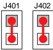
**Figure 16: Jumpers to enable the audio codec**
