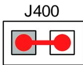
Figure 14: Jumper setting to use Bluetooth over USB
