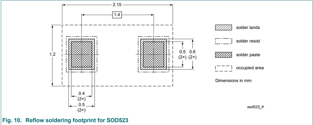
Fig. 10. Reflow soldering footprint for SOD523
