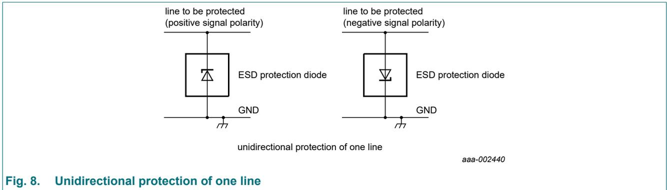
Fig. 8. Unidirectional protection of one line
