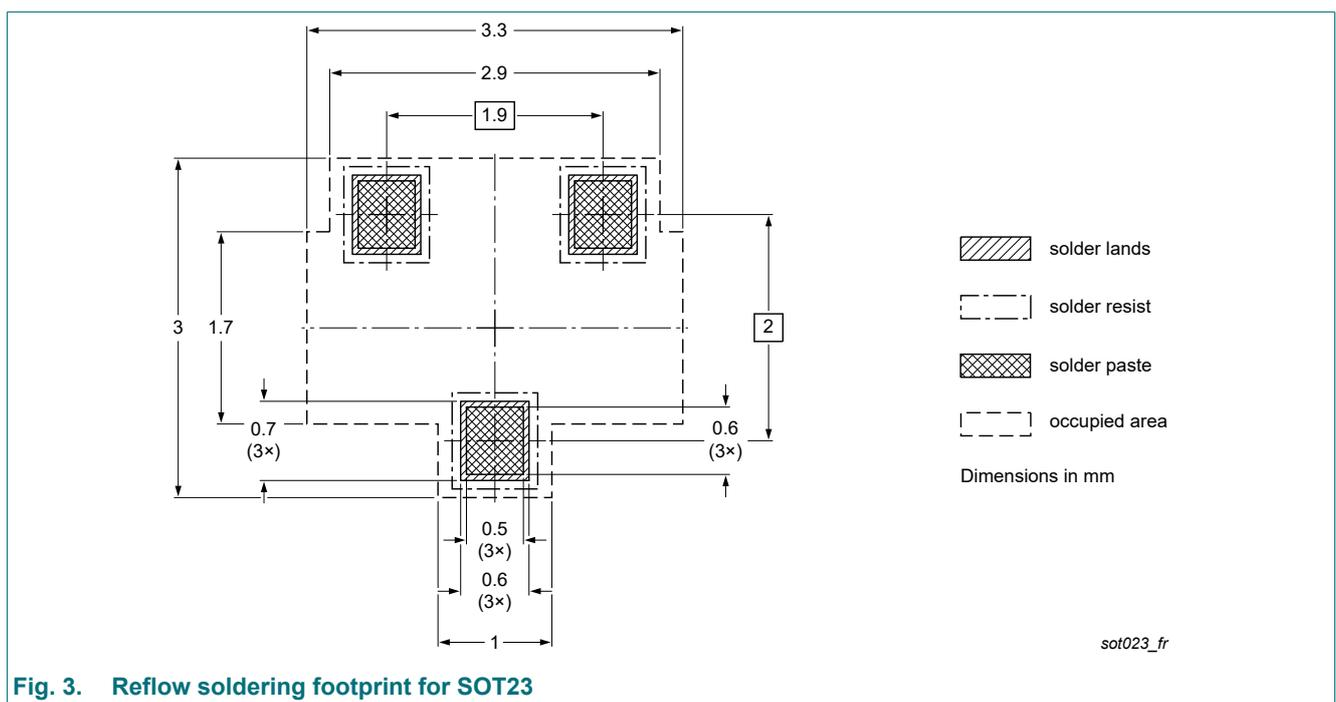
Fig. 3. Reflow soldering footprint for SOT23
