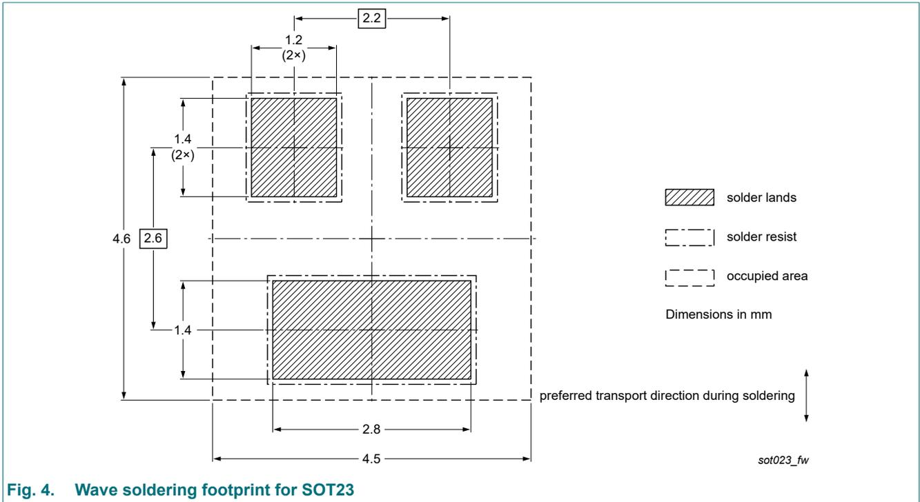
Fig. 4. Wave soldering footprint for SOT23
