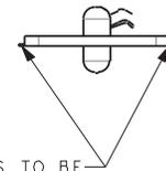
ALL TAILS TO BE WITHIN 0.10 MAX COPLANARITY TOLERANCE
