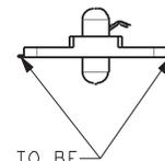
ALL TAILS TO BE WITHIN 0.10 MAX COPLANARITY TOLERANCE
