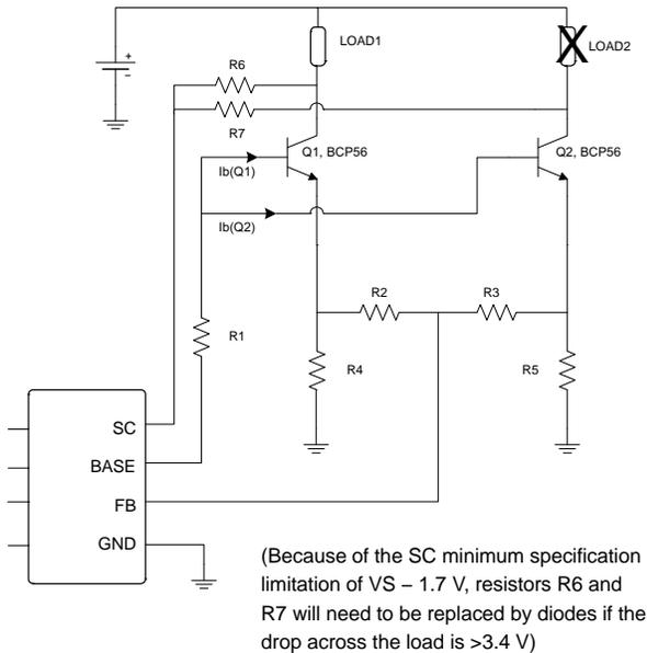
(Because of the SC minimum specification limitation of VS – 1.7 V, resistors R6 and R7 will need to be replaced by diodes if the drop across the load is >3.4 V)
