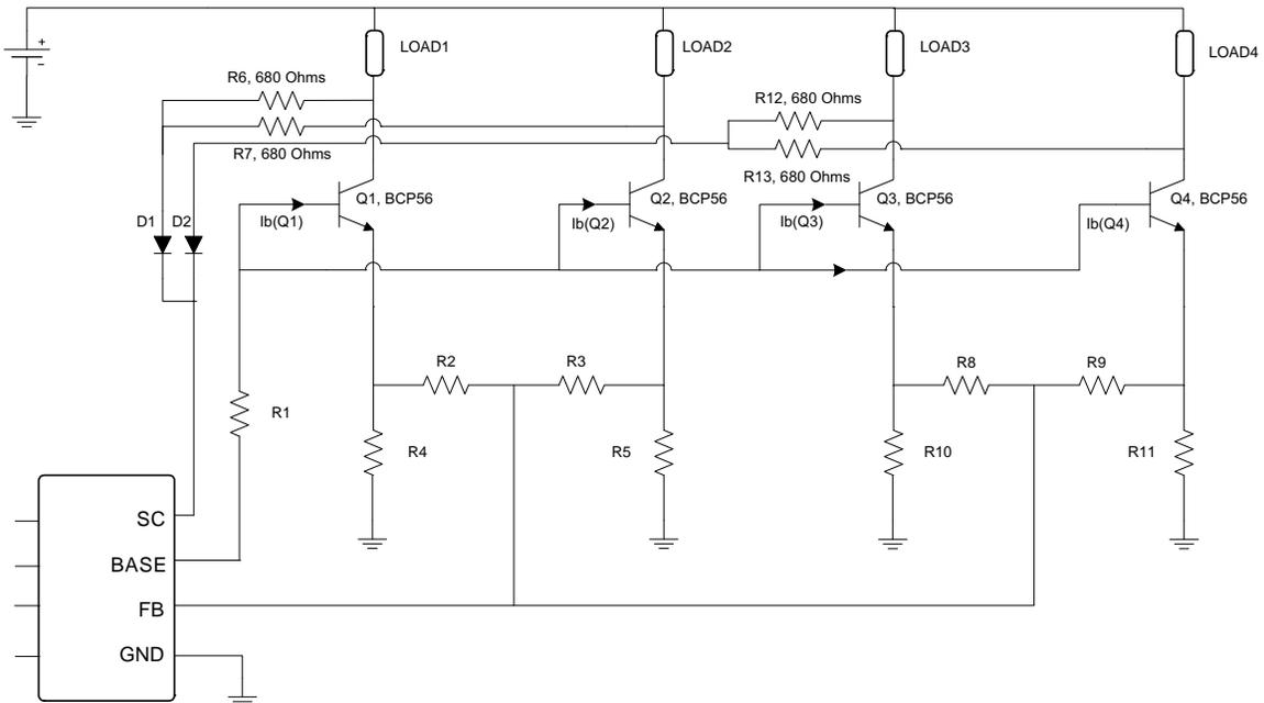
Figure 14. Saving Two Diodes for Short Circuit Protection
