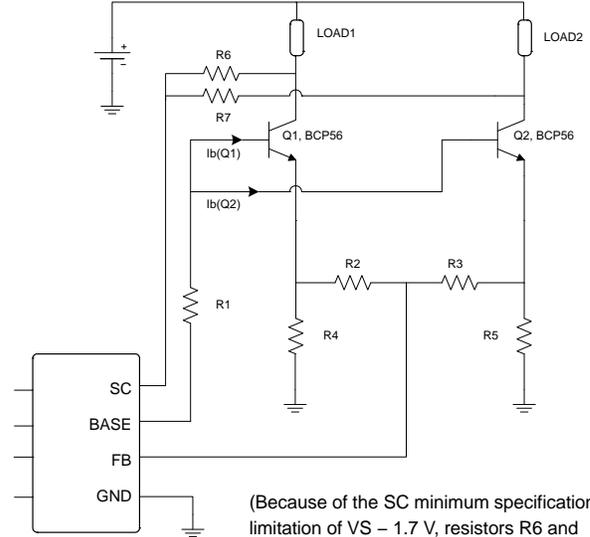
(Because of the SC minimum specification limitation of VS – 1.7 V, resistors R6 and R7 will need to be replaced by diodes if the drop across the load is >3.4 V)
