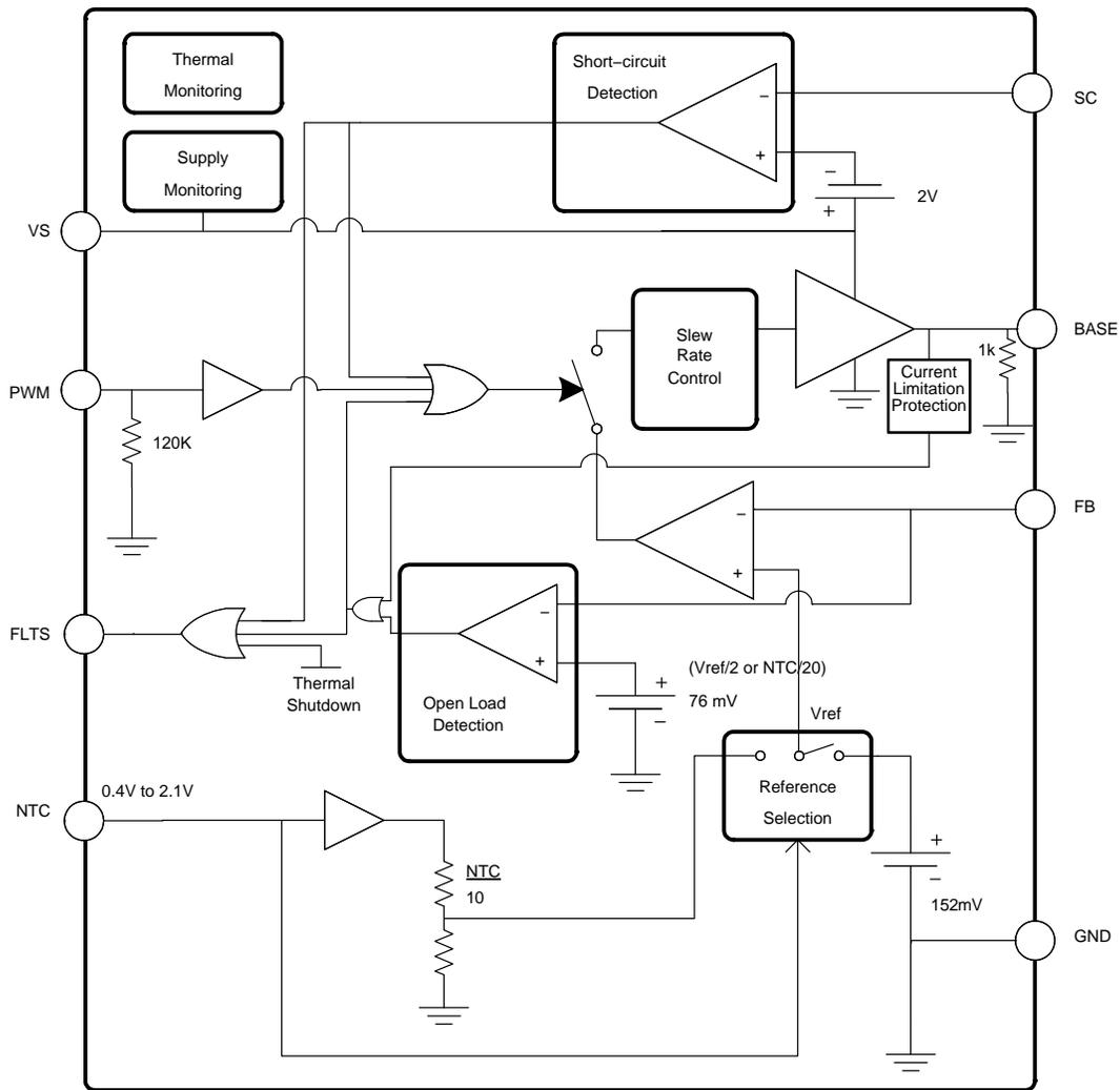
Figure 3. Block Diagram
