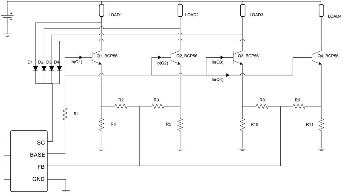
Figure 13. Short Circuit Detection with 4 or more Channels
