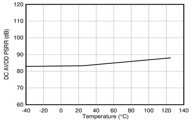
**Figure 6-13. DC AVDD PSRR vs Temperature**
