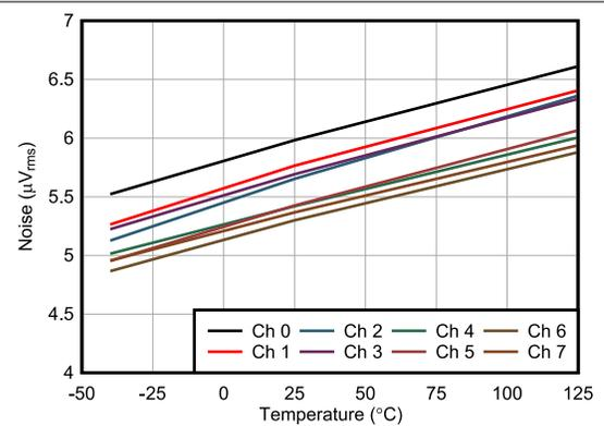
**Figure 6-15. Noise vs Temperature**
