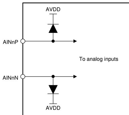
Figure 8-1. Input ESD Protection Circuitry
