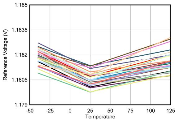
Figure 6-24. Internal Reference Voltage Temperature Drift
