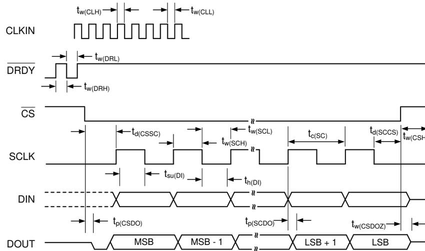
NOTE: SPI settings are CPOL = 0 and CPHA = 1.  $\overline{CS}$  transitions must take place when SCLK is low.
