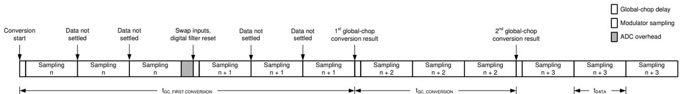
Figure 8-16. Conversion Timing With Global-Chop Mode Enabled
