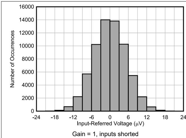
Figure 6-16. Single Device Noise Histogram at 4 kSPS
