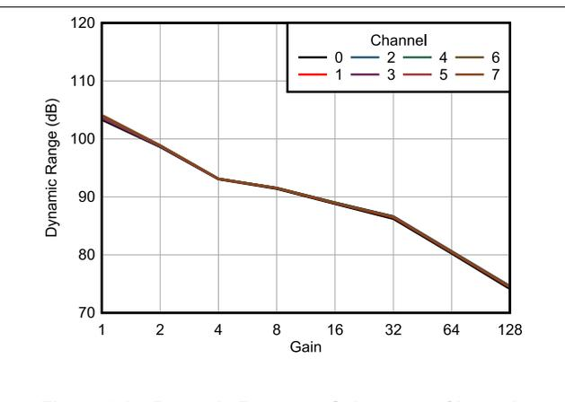
Figure 6-19. Dynamic Range vs Gain across Channels
