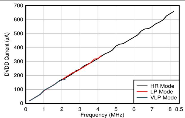
Figure 6-27. DVDD Current vs CLKIN Frequency
