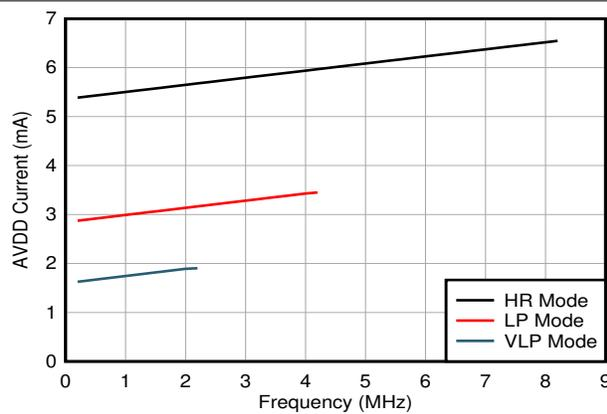
Figure 6-26. AVDD Current vs CLKIN Frequency
