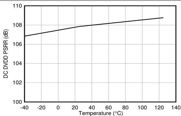
**Figure 6-14. DC DVDD PSRR vs Temperature**
