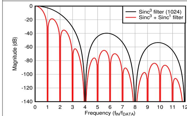
Figure 8-6. Digital Filter Response for OSR = 1024 and OSR = 4096
