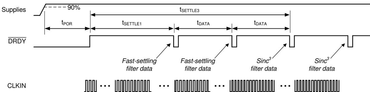
**Figure 8-14. Fast Startup Behavior and Settling Times**
