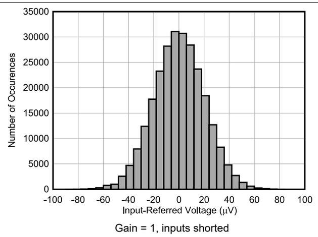
Figure 6-17. Single Device Noise Histogram at 32 kSPS
