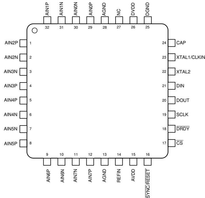
**Figure 5-1. PBS Package, 32-Pin TQFP (Top View)**
