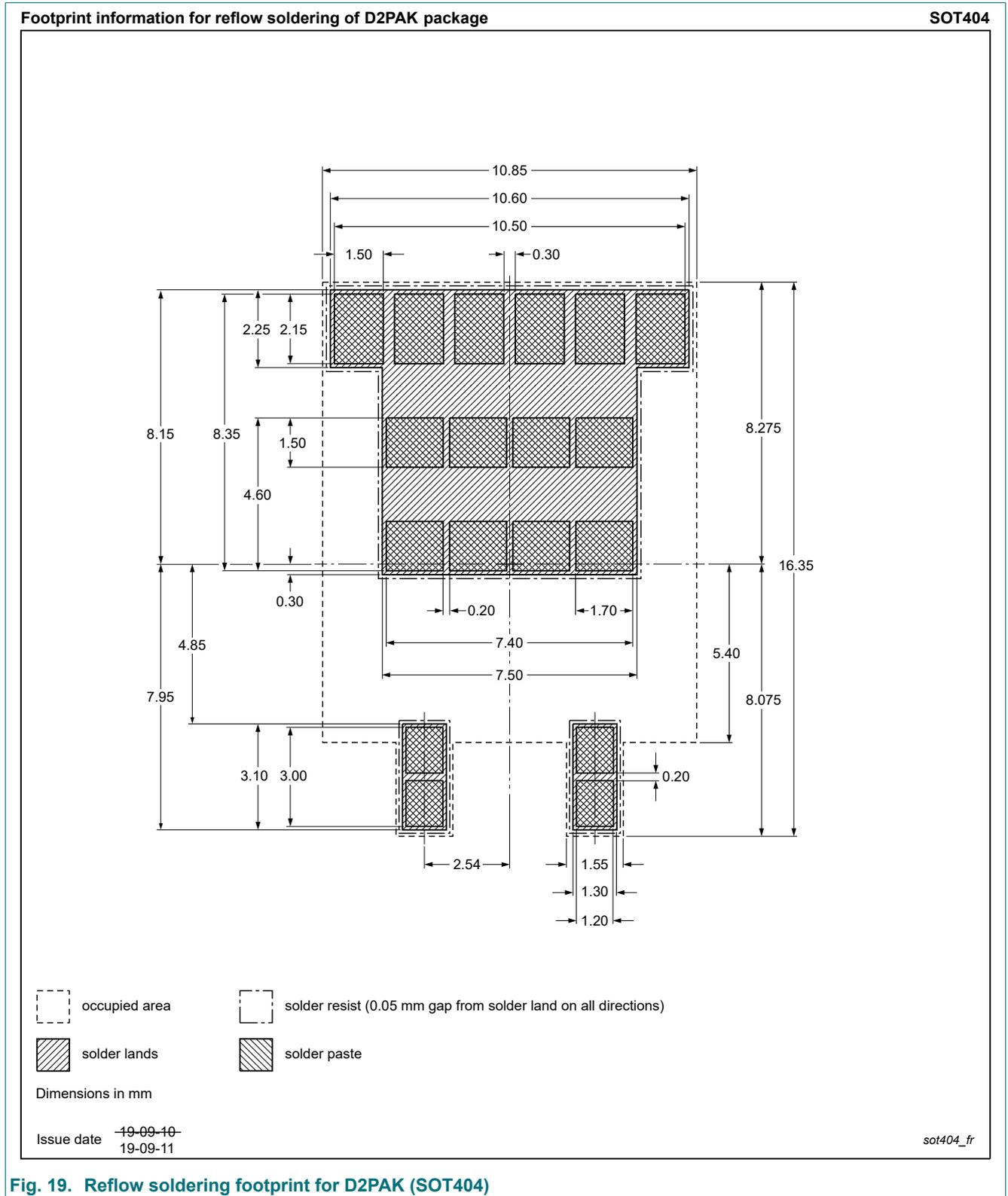
Fig. 19. Reflow soldering footprint for D2PAK (SOT404)
