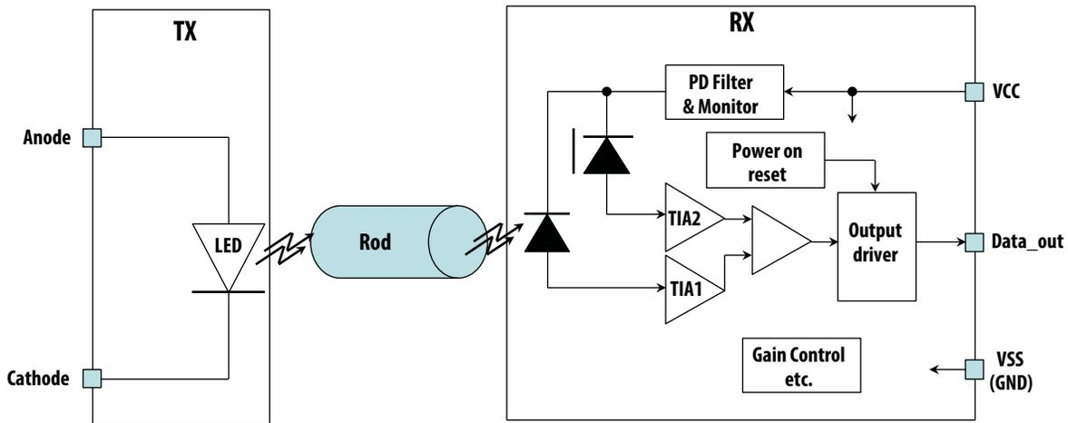
The Rx Data\_out signal is inverted which means that light\_on will lead to Data\_out low.
