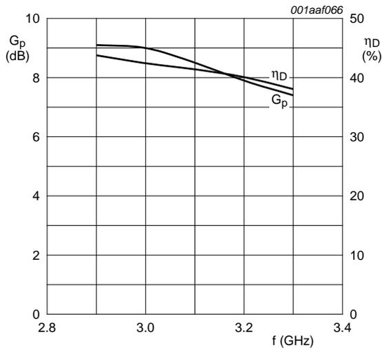
$V_{DS} = 32$  V;  $I_{Dq} = 20$  mA;  $t_p = 200$   $\mu$ s;  $\delta = 12$  %;
