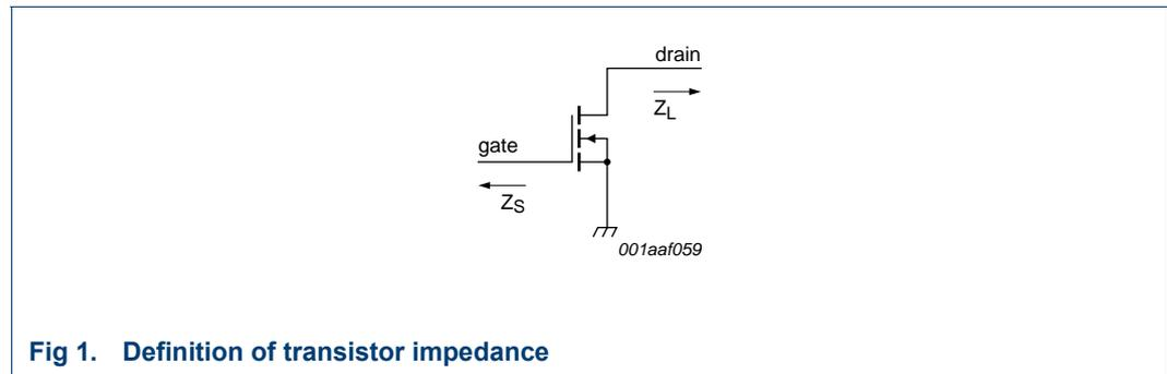
Fig 1. Definition of transistor impedance
