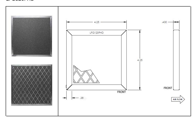
Orion Fans high density air filters offer low pressure drop, fire resistance and the ability to capture large amounts of airborne dust in industrial enclosure applications. Designed for use in equipment where permanent, cleanable filters are most appropriate, these filters are ideal in networking, telecom and communications enclosures.
