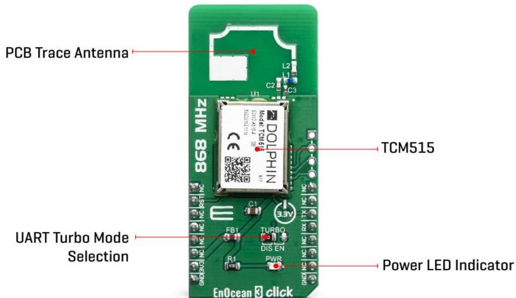
The TCM 515 can work in three functional modes: Telegram Reception, Telegram Transmission, Low Power Sleep.
