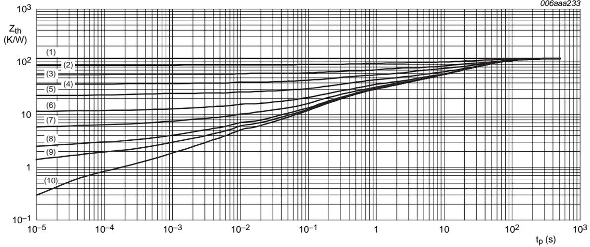
Mounted on FR4 printed-circuit board; mounting pad for collector 1 cm<sup>2</sup>.
