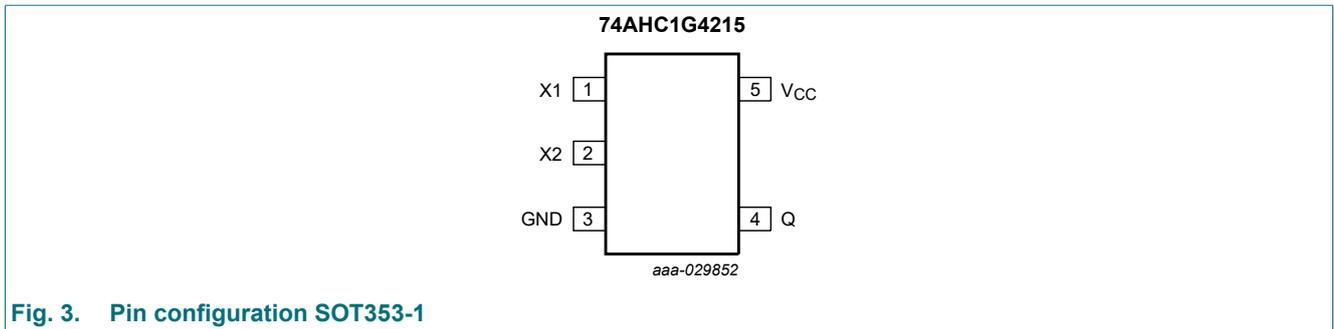
Fig. 3. Pin configuration SOT353-1
