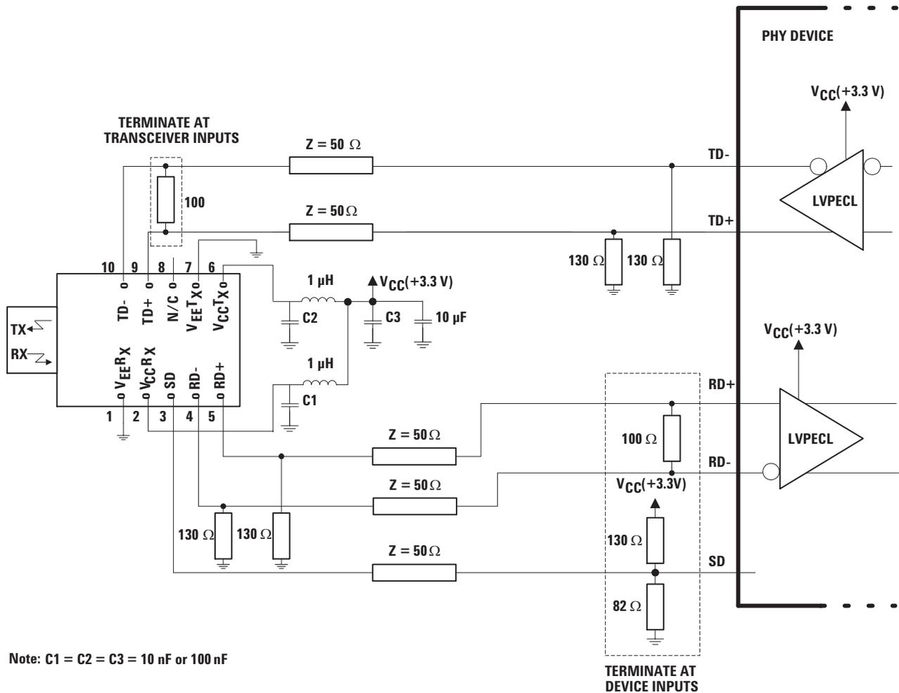
Figure 7. Recommended Decoupling and Termination Circuits
