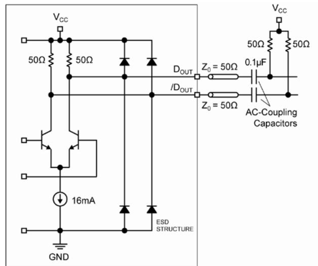
Figure 3. Output Structure
