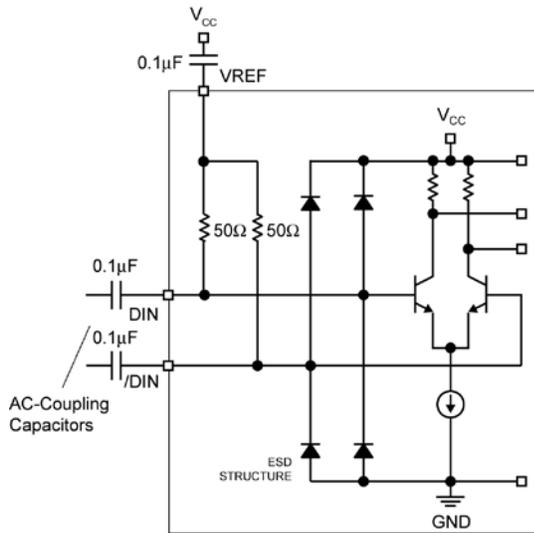
Figure 2. Input Structure
