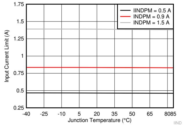
**Figure 7-10. Input Current Limit vs Junction Temperature**
