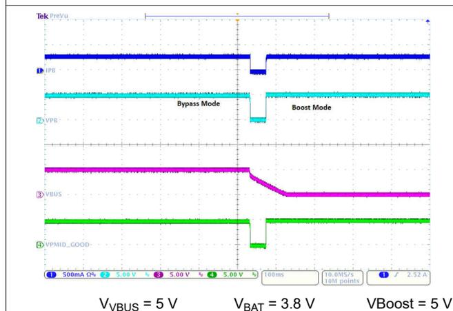
**Figure 9-4. VBUS Unplugged with Boost Mode Enabled**
