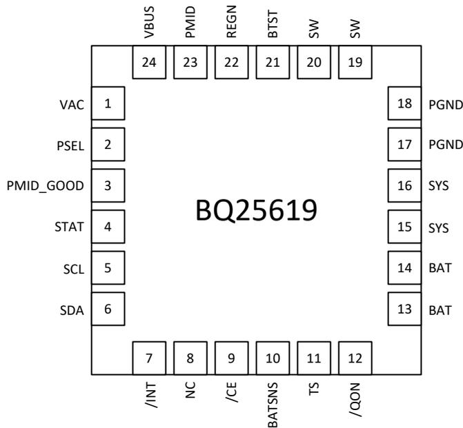
Figure 6-2. BQ25619 RTW Package 24-Pin WQFN Top View
