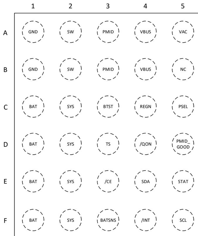
Figure 6-1. BQ25618 YFF Package 30-Pin WCSP Top View
