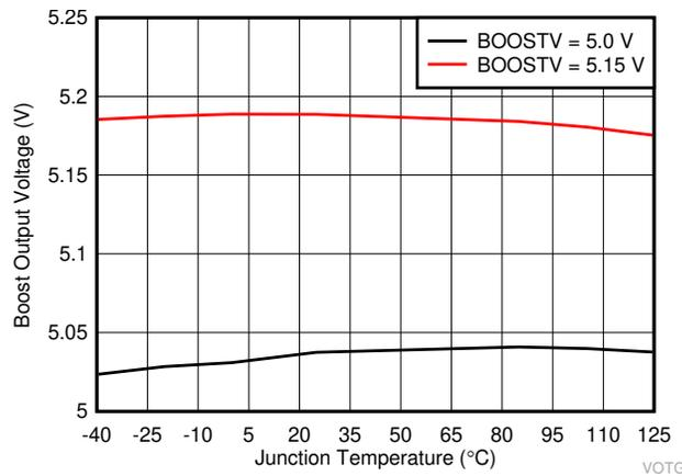
**Figure 7-11. Boost Output Voltage vs Junction Temperature**
