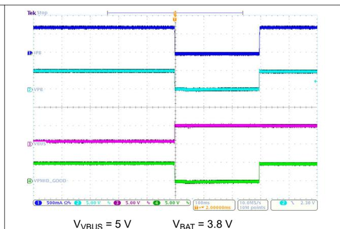
**Figure 9-3. VBUS Plugged In with Boost Mode Enabled**
