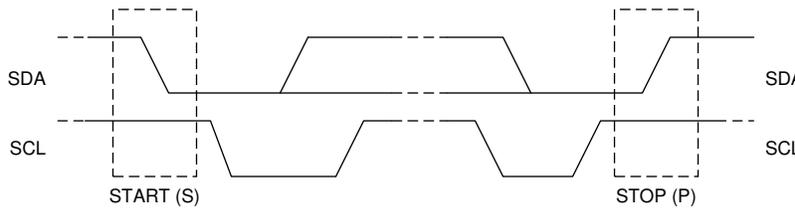
**Figure 8-8. TS START and STOP conditions**
