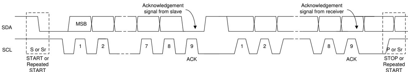
**Figure 8-9. Data Transfer on the I<sup>2</sup>C Bus**
