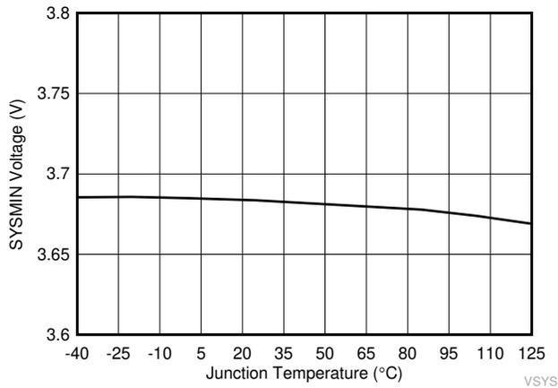
**Figure 7-9. SYSMIN Voltage vs Junction Temperature (VSY set at 3.5 V)**
