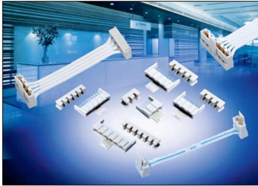
KYOCERA AVX developed the 9159 Series of SMT connectors for co-planar PCB mating for the challenging Solid State Lighting (SSL) market. These connectors needed to be small, low in height, carry up to 5 Amps/contact, and then function up to 125°C for extended periods. This application has been very unique to the SSL market where PCB's are stacked end-to-end to create linear strip lighting in everything from office to transportation applications.
