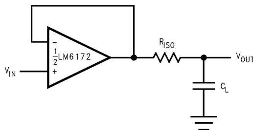
**Figure 43. Isolation Resistor Used to Drive Capacitive Load**
