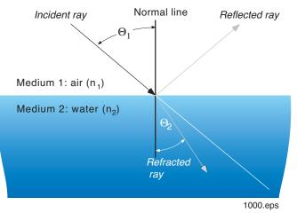
Figure 4. Ray of light traveling through two materials
