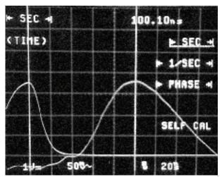
Figure 7. Oscilloscope display showing approximate positions of the reference pulse and the received pulse delayed through 20 meters of fiber.
