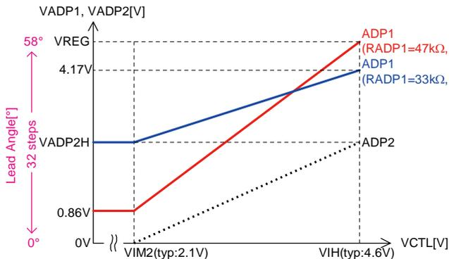
4. When the lead angle is not adjusted
