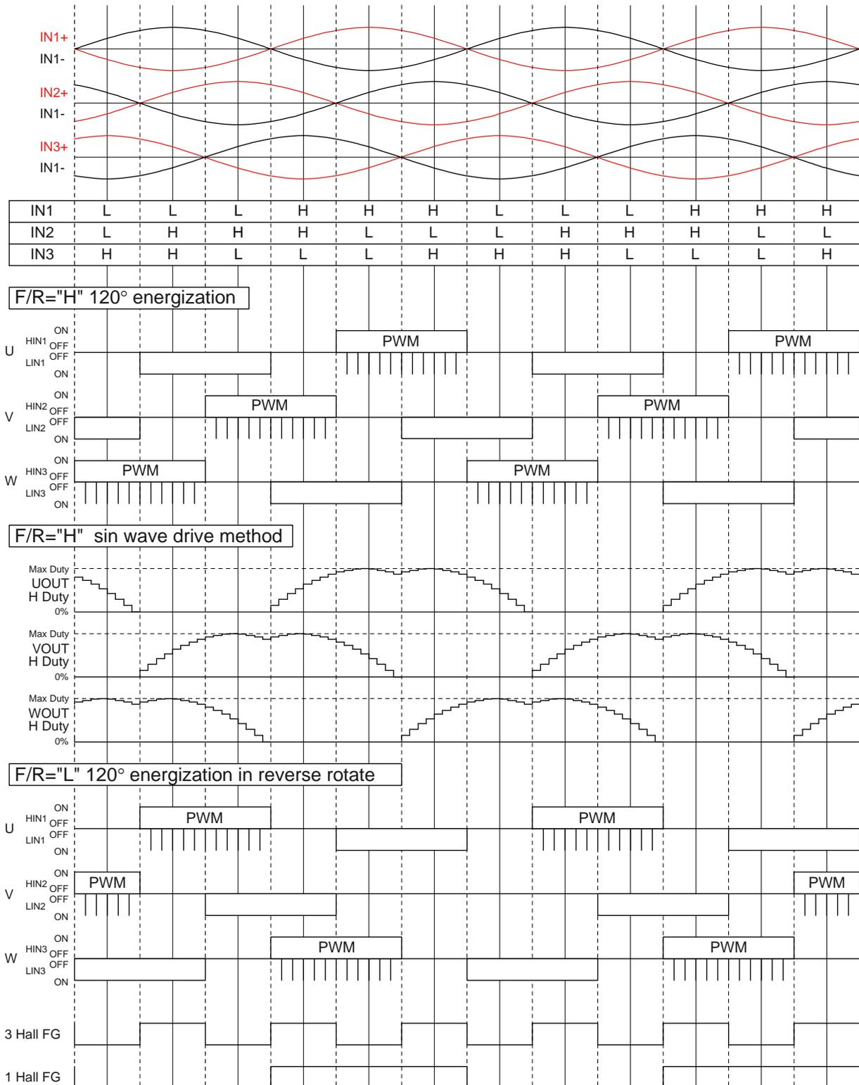
The energization is switched to 120° when 3 Hall FG frequency is 5.15Hz (typ) or lower
