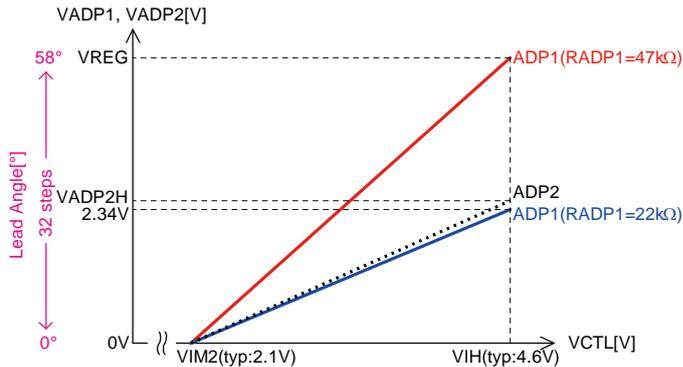
2. The ADP2 pin rise can be halted (a limit on the lead angle adjustment can be set by means of the CTL voltage) by setting DPL (pin 10).
