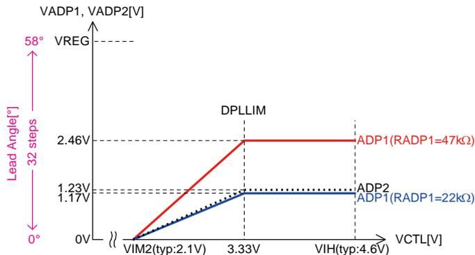
3. The offset and slope can be adjusted as desired by setting RADP1 and RADP12 of ADP1 (pin 15). (It is also possible to set a limit on the lead angle
