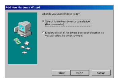
Now a new driver has to be installed. You can specify the location of the driver files in the lower entry field.
