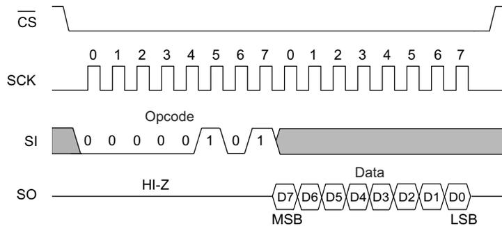
Figure 10. WRSR Bus Configuration (WREN not shown)
