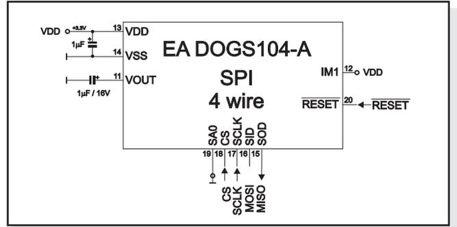
To guarantee an error-free functionality and initialization of display it is recommended to operate the reset input actively. This can be done via microcontroller port or external circuit. Here's an application example:
