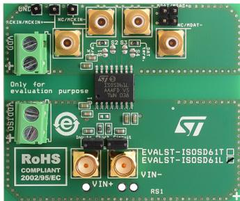
**Figure 2. EVALST-ISOSD61T board**
