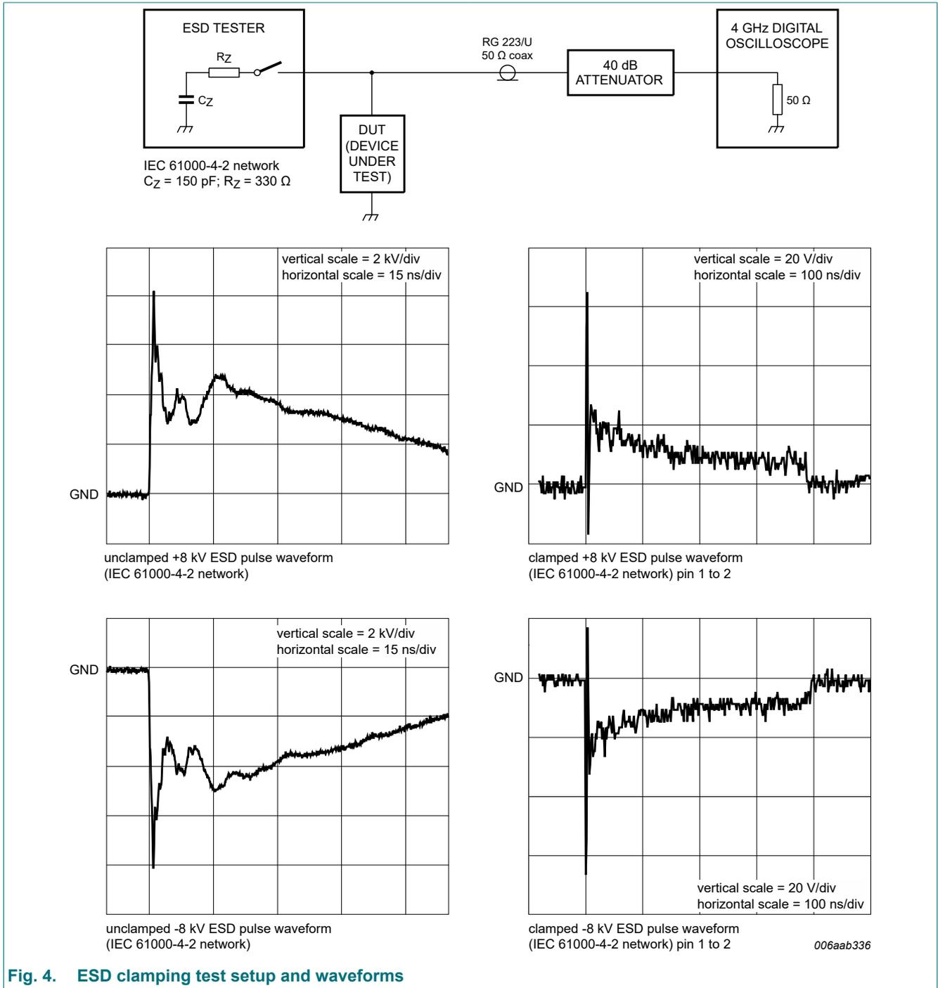
Fig. 4. ESD clamping test setup and waveforms
