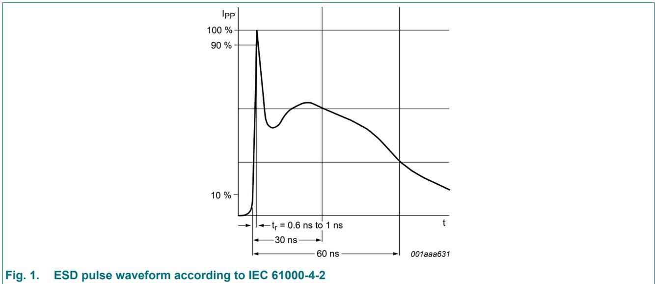
**Fig. 1. ESD pulse waveform according to IEC 61000-4-2**
