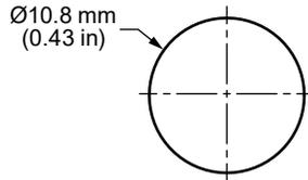
Figure 2. ANT-916-WRT Series Antenna Recommended Enclosure Mounting Dimensions
