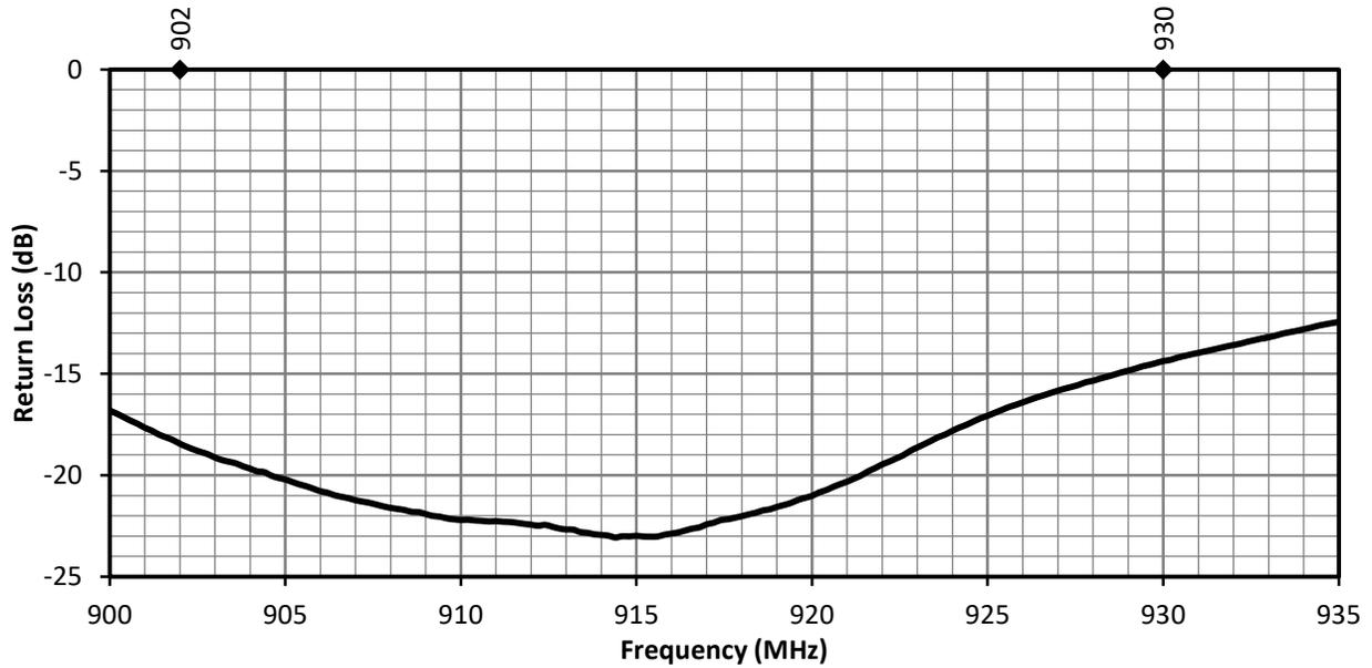
Figure 13. ANT-916-WRT Return Loss, Center of Ground Plane
