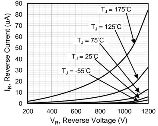
Fig.2 Reverse Characteristics
