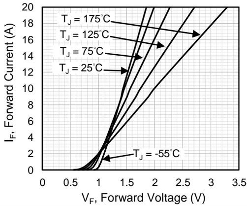
Fig.1 Forward Characteristics
