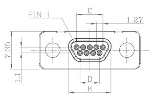
USE ABOVE FRONT FACE DIMENSIONS FOR PCB LAYOUT DESIGN.  $\emptyset 0.8 \text{mm}$  HOLE SIZE IS RECOMMENDED.
