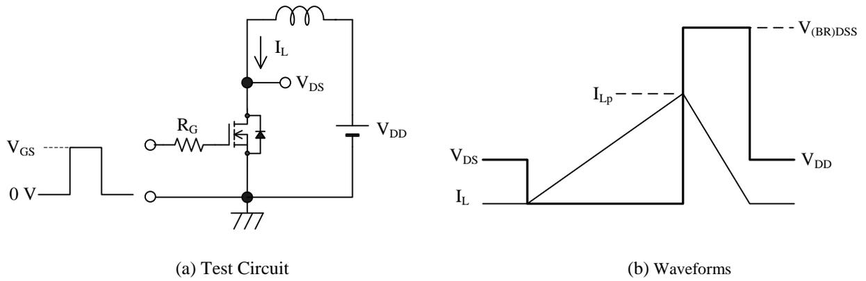
Figure 1 Unclamped Inductive
