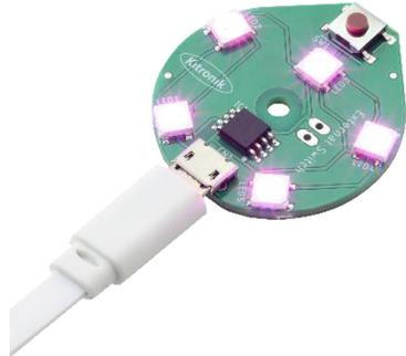
The board has 4 patterns, selected by pressing the button to step through them. There is an additional off position after the 4<sup>th</sup> pattern:
