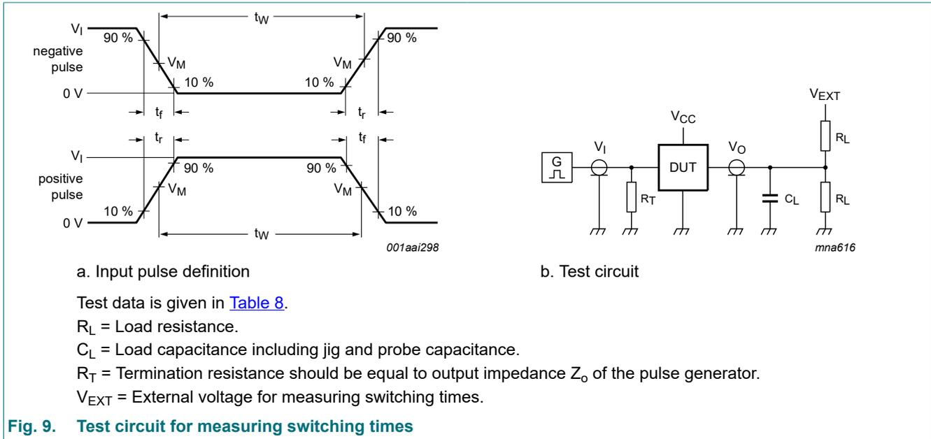
Fig. 9. Test circuit for measuring switching times
