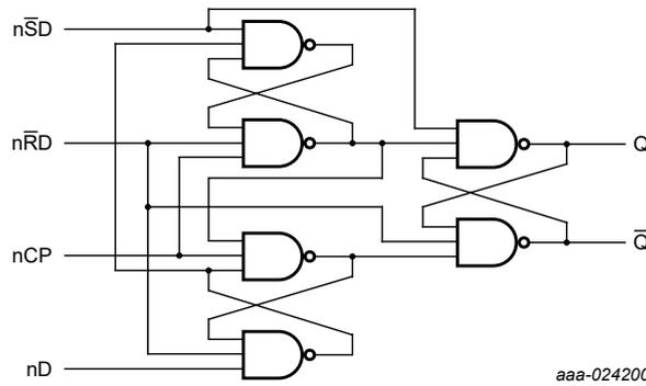
Fig. 3. Logic diagram for one flip-flop
