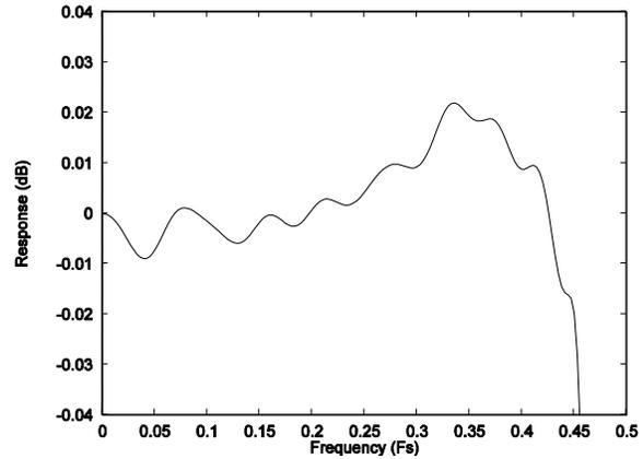
Figure 29 ADC Digital Filter Frequency Response – Type 0
