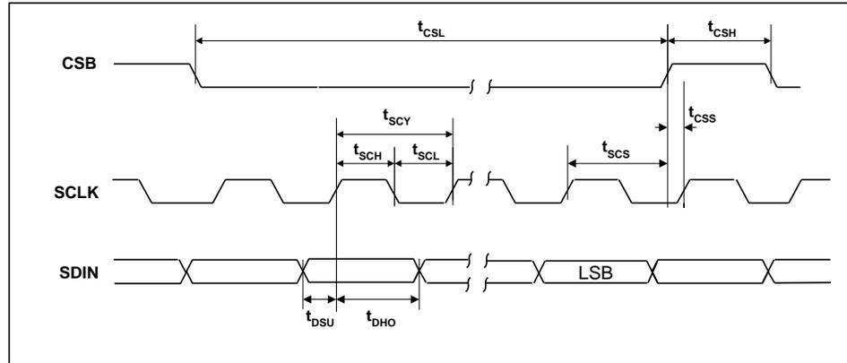
**Figure 4 Control Interface Timing – 3-Wire Serial Control Mode**
