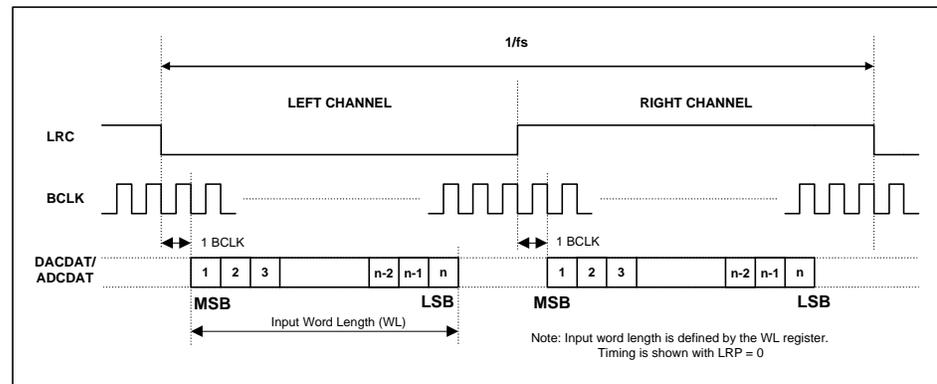
**Figure 13 I<sup>2</sup>S Justified Audio Interface (assuming n-bit word length)**
