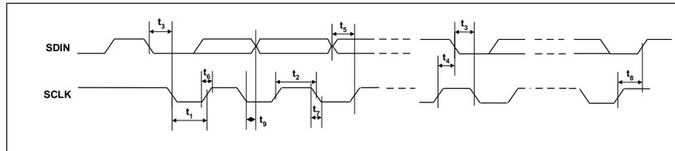
**Figure 5 Control Interface Timing – 2-Wire Serial Control Mode**
