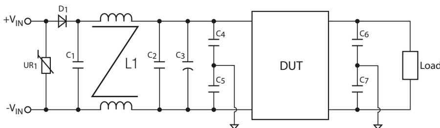
It is recommended to add UR1, D1 and C1 in railway application. C1, L1, C2 and C3 can be modified for required EMI standards. To meet EN61000-4-2, module case should be earth grounded. We offer independent case pin option on request.
