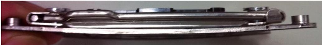
It is normal state for ILM curved when lever is closed. The reason is lever will provide a closing force on load plate and a hook-up force on frame.
