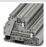
Multi-level terminal block, Connection method: Screw connection, Cross section: 0.14 mm² - 6 mm², AWG: 26 - 10, Width: 6.2 mm, Height: 60.1 mm, Color: gray, Mounting type: NS 35/7,5, NS 35/15
