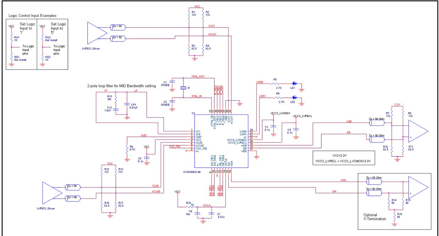
Figure 7. ICS843002I-40 Schematic Example
