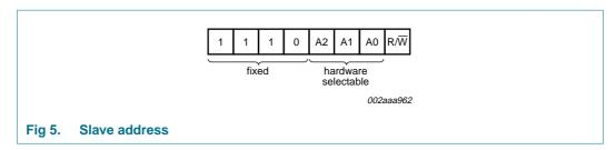
The last bit of the slave address defines the operation to be performed. When set to logic 1 a read is selected, while a logic 0 selects a write operation.
