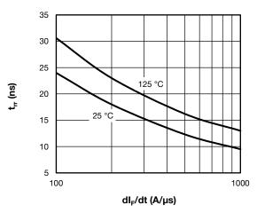
Fig. 6 - Typical Reverse Recovery Time vs. dl<sub>F</sub>/dt
