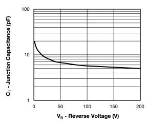
Fig. 3 - Typical Junction Capacitance vs. Reverse Voltage
