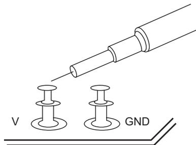
**Figure 4. Voltage Ripple Test**
