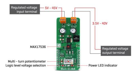
The output voltage can be adjusted by a precise multi-turn potentiometer. This potentiometer allows adjustment of the output voltage level by changing the resistance value of the voltage divider that feeds part of the output voltage back to the FB pin of the MAX17536. Since the potentiometer is a mechanical component, it will allow the output voltage to remain the same, even after the power cycle.
