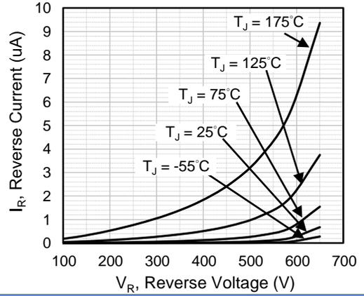
Fig.2 Reverse Characteristics
