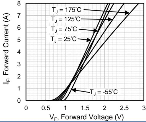
Fig.1 Forward Characteristics
