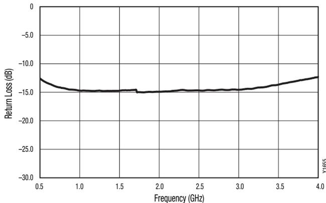
Figure 6. RF2 Return Loss (Isolation State) vs Frequency
