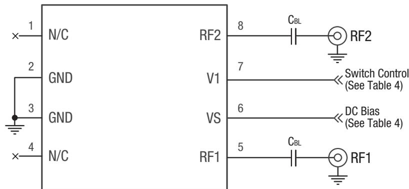
*Note: C<sub>BL</sub> = 47 pF for >500 MHz operation; 220 pF for operation down to 50 MHz. Higher values recommended for lower frequency operation. Exposed paddle must be grounded.*
