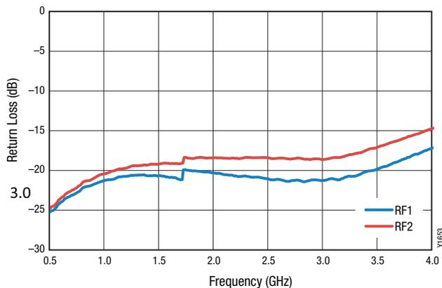
Figure 4. Return Loss (Insertion Loss State) vs Frequency
