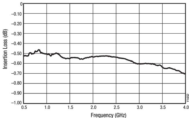
Figure 3. RF1 to RF2 Insertion Loss vs Frequency
