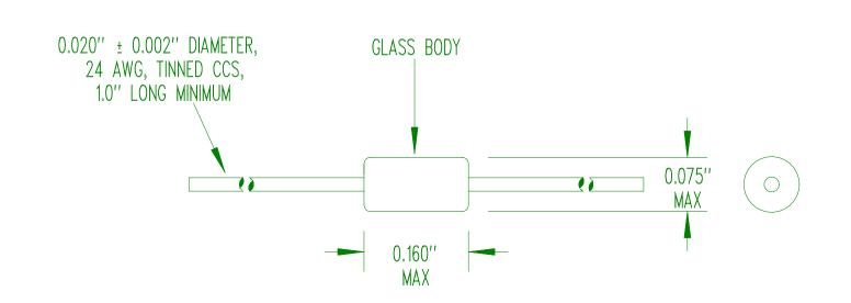
RESISTANCE @  $+25^{\circ}\text{C} = 30,000 \ \Omega \pm 5\%$ RESISTANCE/TEMPERATURE CURVE = "J"
