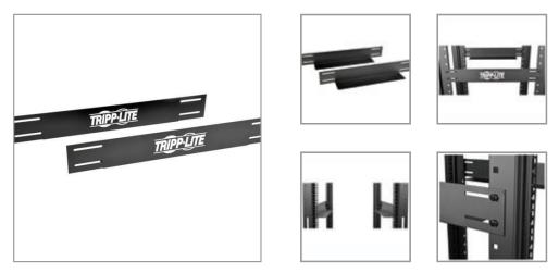
Installs on the outside edges of your 4-post rack's vertical mounting rails as extra support for a rack-mount UPS system or other networking or power protection equipment 17.5 in. wide.
