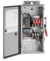
Slim Line Pump Control Panel NEMA size 1 Three phase full voltage Solidstate overload relay OLR amp range 3-12A 460VAC 60Hz Coil 30A fusible disconnect 30A/600V fuse clip 1NC / 1NO auxiliary contacts HOA Sel. Sw. <(>&<)> Start/Stop 3-point power terminal block 3-point control terminal block 3-point ground lug Enclosure NEMA type 3/3R Weather proof outdoor use
