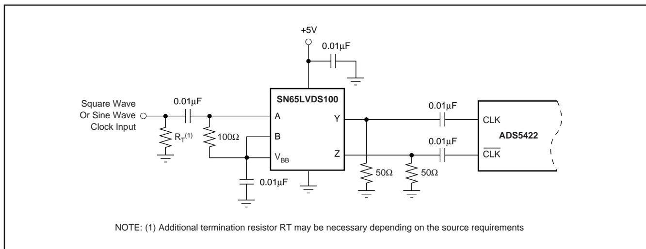
FIGURE 13. Differential Clock Driver Using an LVDS Translator.
