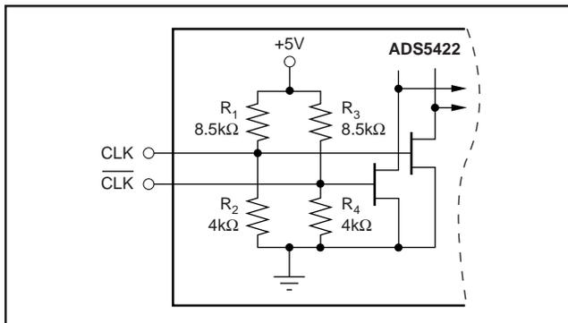
FIGURE 10. The Differential Clock Inputs are Internally Biased.
